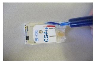
Insert syringe tip into the sample well, then slowly twist and push the plunger downwards until the sample reaches fill mark (see diagram in red on cartridge)
