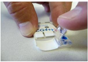
Once blood has been filled up to the appropriate mark, flip the closure across to seal the sample well, pushing down on the clear plastic tab section of the closure
